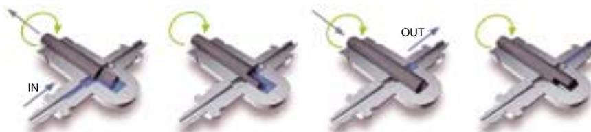
The plunger moves in and out as it rotates. As the cut-out section on the end of the plunger rotates, the suction and discharge ports are alternately opened and closed such that fluid is taken in and discharged.
